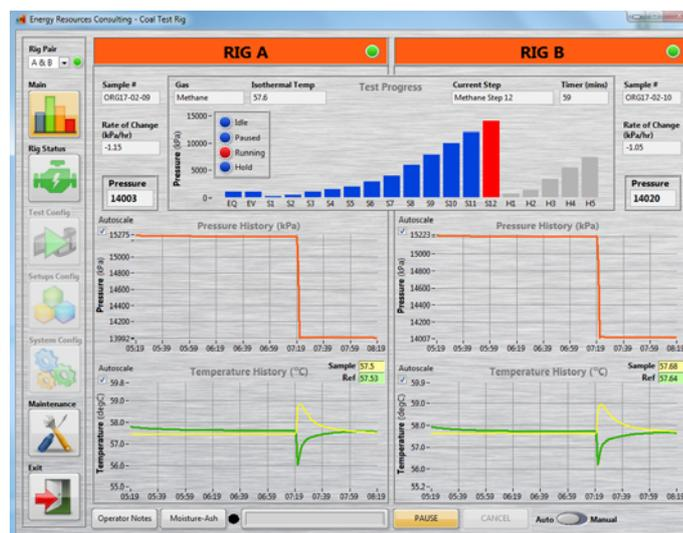
Screen capture during a live run showing pressure and temperature within each cell in real time as well as the pressure step within the overall run
