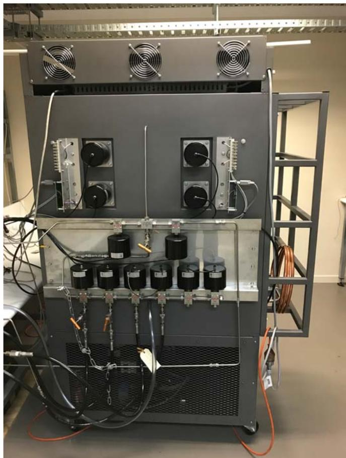
*Rear view of air bath model showing air actuated valves that control gas flows*
