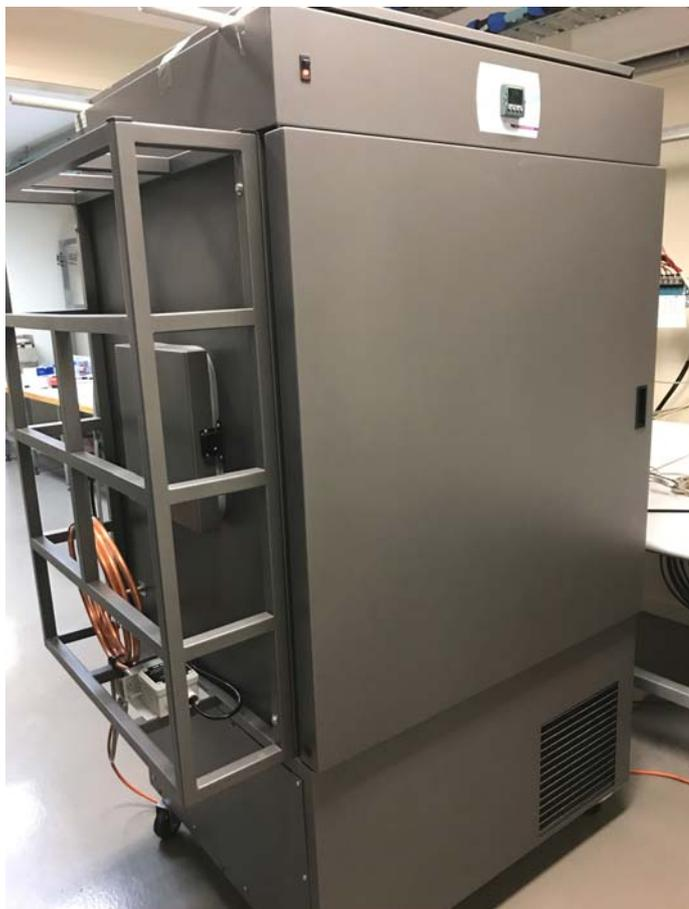
*Front view of air bath model showing safety systems of blow-out panel with cage and hydrocarbon gas monitoring system*
