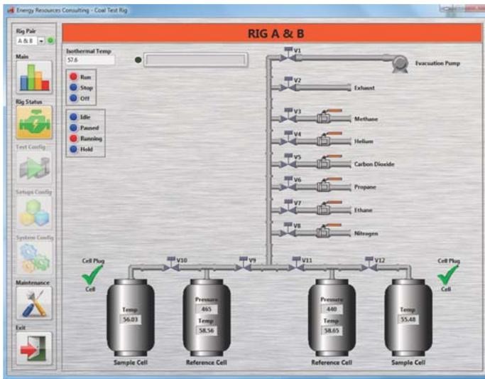
Screen capture during a live run showing status of valves (open or closed) and pressure and temperature within cells
