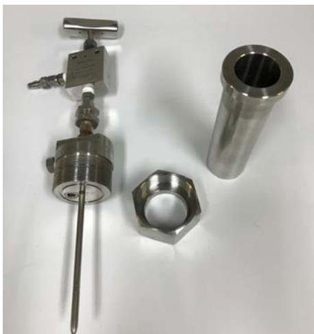
Custom built pressure vessels incorporate a thermocouple to measure temperature inside the cell
